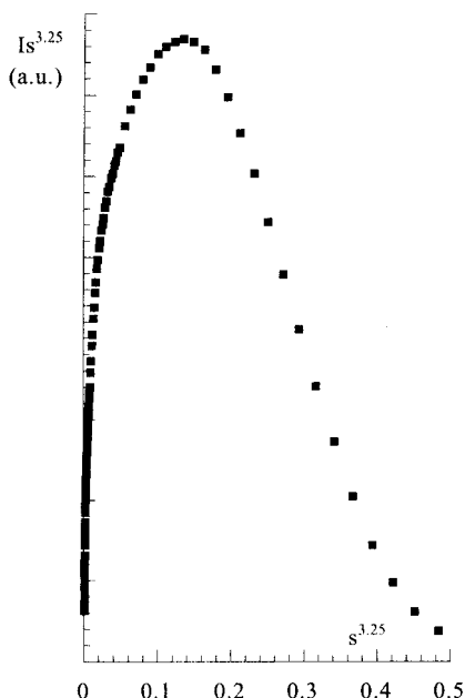
Figure 2. Plot of I s^\alpha ( \alpha = 3.25 ) vs s^\alpha for PIP-S-Sr-8000. The maximum at 0.14 in the Porod region ( s = 0.55 \text{ nm}^{-1} ) is the signature of a angulous contribution to the tail-end of the scattering curve.
